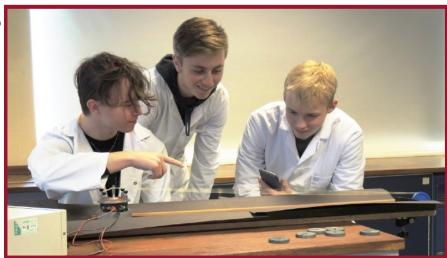
adjusting the vibration generator. We found that the higher the tension the higher the natural frequency, as every guitar player knows. Second we placed a fixed weight of 2.45 Newtons (that is a 250 gram mass) on the end of the string and found how changing the length changed the frequency. We found the longer
